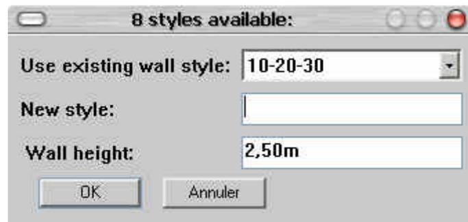
Once you have clicked on the "OK" button, click a first point and a second point. These are the starting and ending points of the axis of the wall basis. Each wall segment is drawn as a group.
